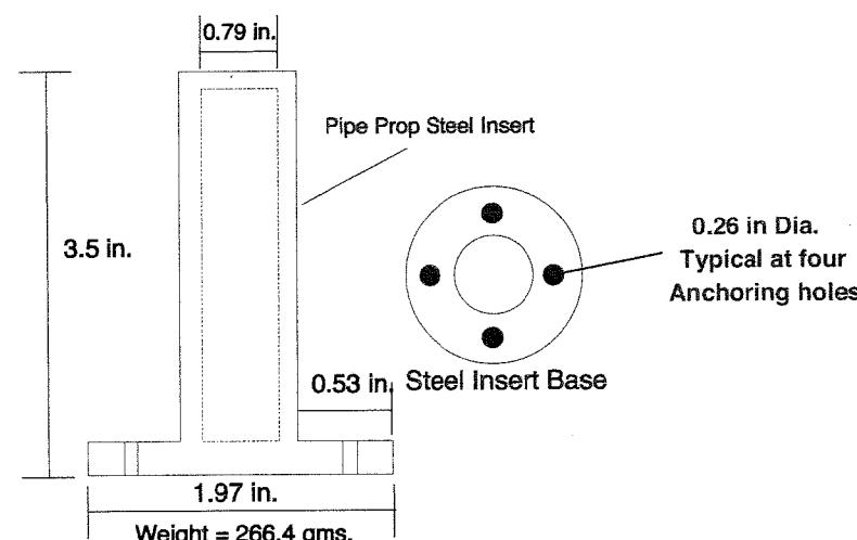
MDA-HZ1 Steel Insert required when supporting electrical conduit
